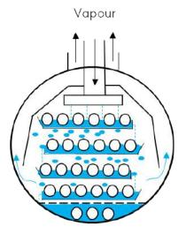
The heat exchanger consists of a steel shell insulated with closed-cell foam material, while the tube bundle is made with copper tubes. The heads can be removed for tube inspection and cleaning. Victaulic couplings on water side (complete with nipple for connection). On the hydraulic connections of the heat exchanger, there are also pipe taps for the differential pressure switch, and wells for the temperature probes.
