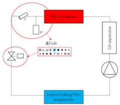
The electronic expansion valve is designed to offer enhanced stability during operation and to maximise the use of evaporation under all load conditions. This also acts as shut-off valve on the liquid line, thereby preventing hazardous refrigerant migrations during compressor stops.
