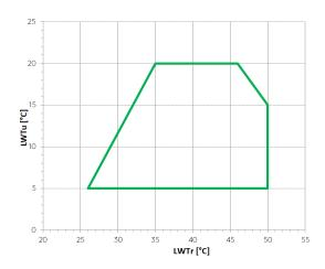
**LWTs:** water outlet temperature from the source-side heat exchanger **LWTu:** water outlet temperature from the user-side heat exchanger **LWTr:** water outlet temperature from the recovery exchanger
