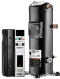
All the units use a hermetic orbiting spiral scroll compressor with brushless motor controlled by a DC inverter. In the models with two or three compressors, this is connected in tandem or trio with hermetic scroll compressors with asynchronous ON/OFF motor.
